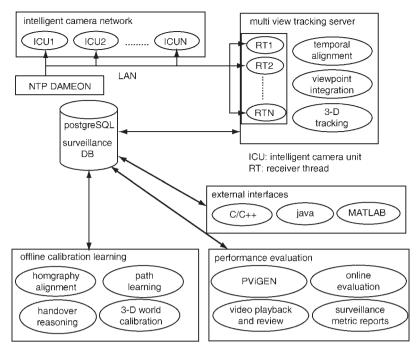
Fig. 4 Architecture of multi-camera surveillance system (from Makris et al. [62])
