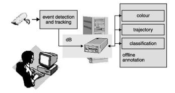
Fig. 8 Architecture of VIGILANT system (from D. Greenhill et al. [32])
