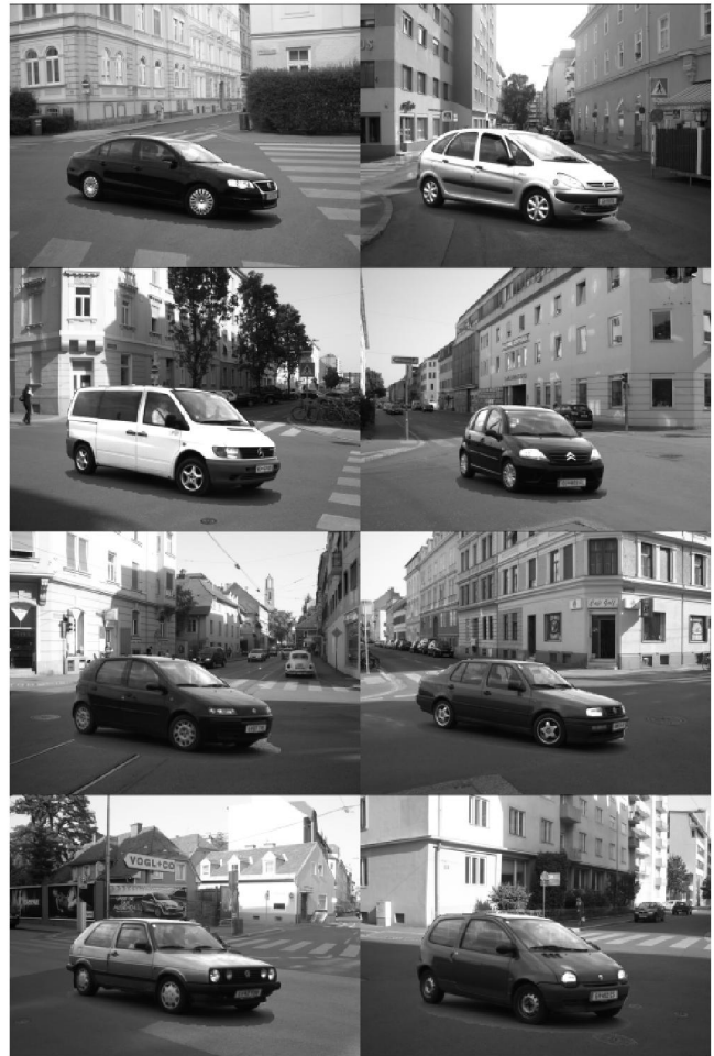
Fig. 3. Projection of various cars onto different backgrounds. We simulate the various levels of background noise by cropping the vehicle out of the images again with a varying border added around the object.
