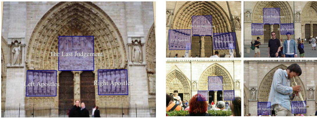
Figure 7: Example of annotation transfer. Three regions were annotated in the photograph on the left; the annotations were automatically transferred to the other photographs, a few of which are shown on the right. Our system can handle partial and full occlusions.
