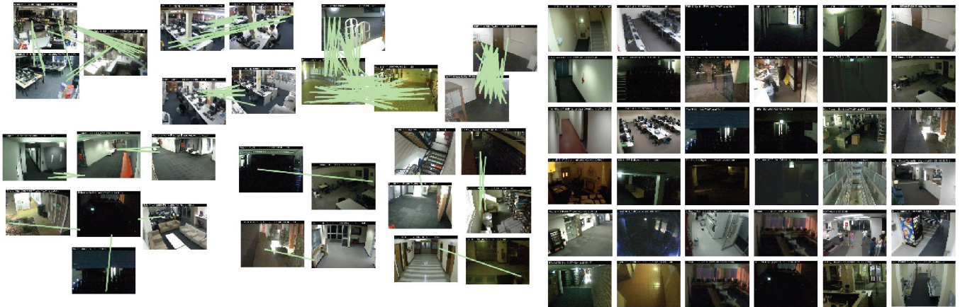
Fig. 2. Video feeds after running exclusion on one hour of footage from cameras spread across a university campus. The cameras are arranged on screen so that related cameras are near each other.
