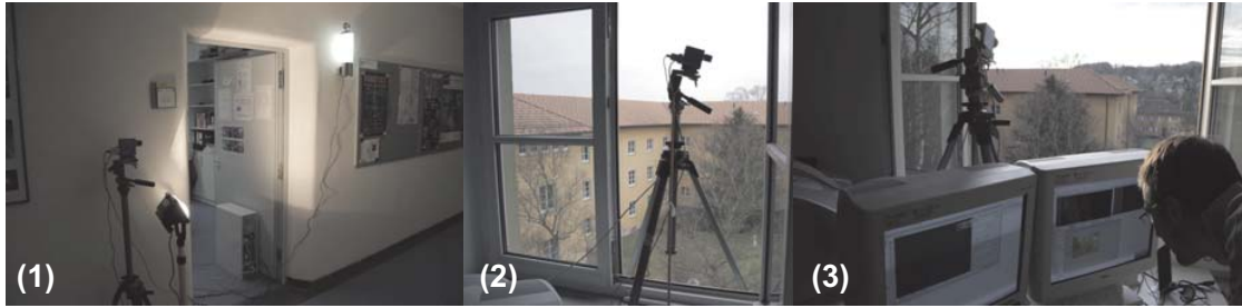
Figure 11. (1) Indoor Setup. Note the smart camera on the tripod, halogen illumination and a webcam on top of a light. (2, 3) Outdoor setup.
