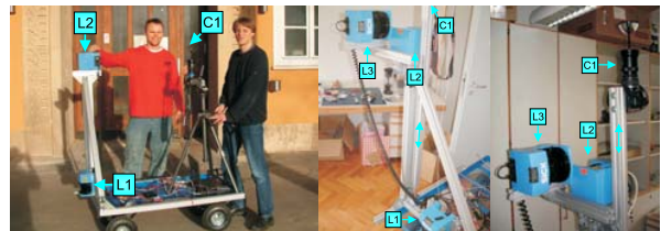
Figure 10. Two setups of our mobile platform. Left: Two Laser scanners L1, L2 and one omnidirectional camera. Center & Right: Three laser scanners L1, L2, L3 and omnidirectional camera closely mounted together.
