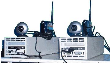
Fig. 4. Two sensor node subsystems with a camera and a wireless bridge. a size of 28.5mm. Two grid patterns can be seen in Fig. 3a attached to two target planes. It is clear that the choice of the grid size directly affect the quality of the calibration. Before performing the experiments with the target mounted robot we used a large grid (13 by 17 squares, see Fig. 5) as a base of comparison for the calibration of the internal parameters.
