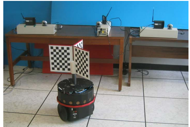
Fig. 1. Three wireless camera nodes and the mobile robot with the target. every time it passes through a camera's field of view. After obtaining a number of images the internal and the external parameters [3] of the camera are estimated. Finally, the 3D pose of the camera is recovered as a function of the pose of the robot for each of the images taken.
