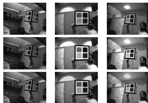
Figure 11: Row 1: Three original views. Row 2: The same three different after deliberate simulated miscalibration of the greyscales. Row 3: The views after evolution of the calibration parameters has completed.
