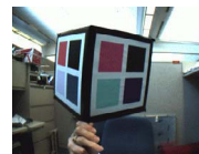
Figure 2: Photograph of the color calibration object.
