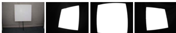
Figure 1: Three out of five camera views of the real calibration object shown on the left.
