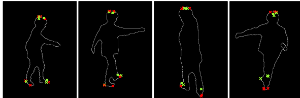
Figure 6. Silhouette images and estimated frontier points (Red: frontier points, which should be visible on the silhouette contours. Green: other frontier points.)
